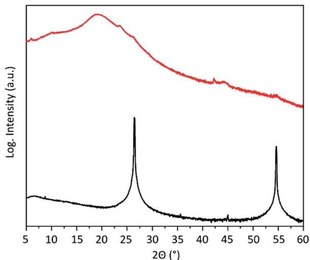
Fig. 4 XRD pattern of the graphite flakes before (black) and after (red) electrochemical exfoliation.
