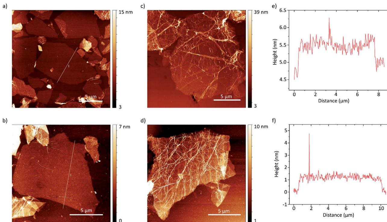
Fig. 5 (a–d) AFM height images of hydrogenated graphene flakes on SiO<sub>2</sub> (300 nm)/Si substrates. The profile lines shown in (a) and (b) are depicted in (e) and (f) respectively.
