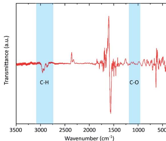
Fig. 3 FTIR spectrum of the graphene flakes. The silicon substrate signal was used for baseline correction giving rise to the peaks in the range below 1700 cm<sup>-1</sup>. The uncorrected spectra for both substrate and the graphene sample are shown in the ESI.† The shaded areas mark the presence of C–H vibrations and the absence of C–O bands.
